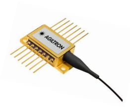
butterfly package. The laser diodes contain a thermoelectric cooler (TEC), and a thermistor to secure high-quality laser performance. The Laser Diodes Wavelength of 495±10nm, Output power: ≥30mW, Pigtail Type: 405-HP(Nufern) fiber with 900um loose tube, 1.0+/-0.1m, FC/APC connector. Our laser products are Telcordia GR-468 qualified and in compliance with RoHS Directives.
